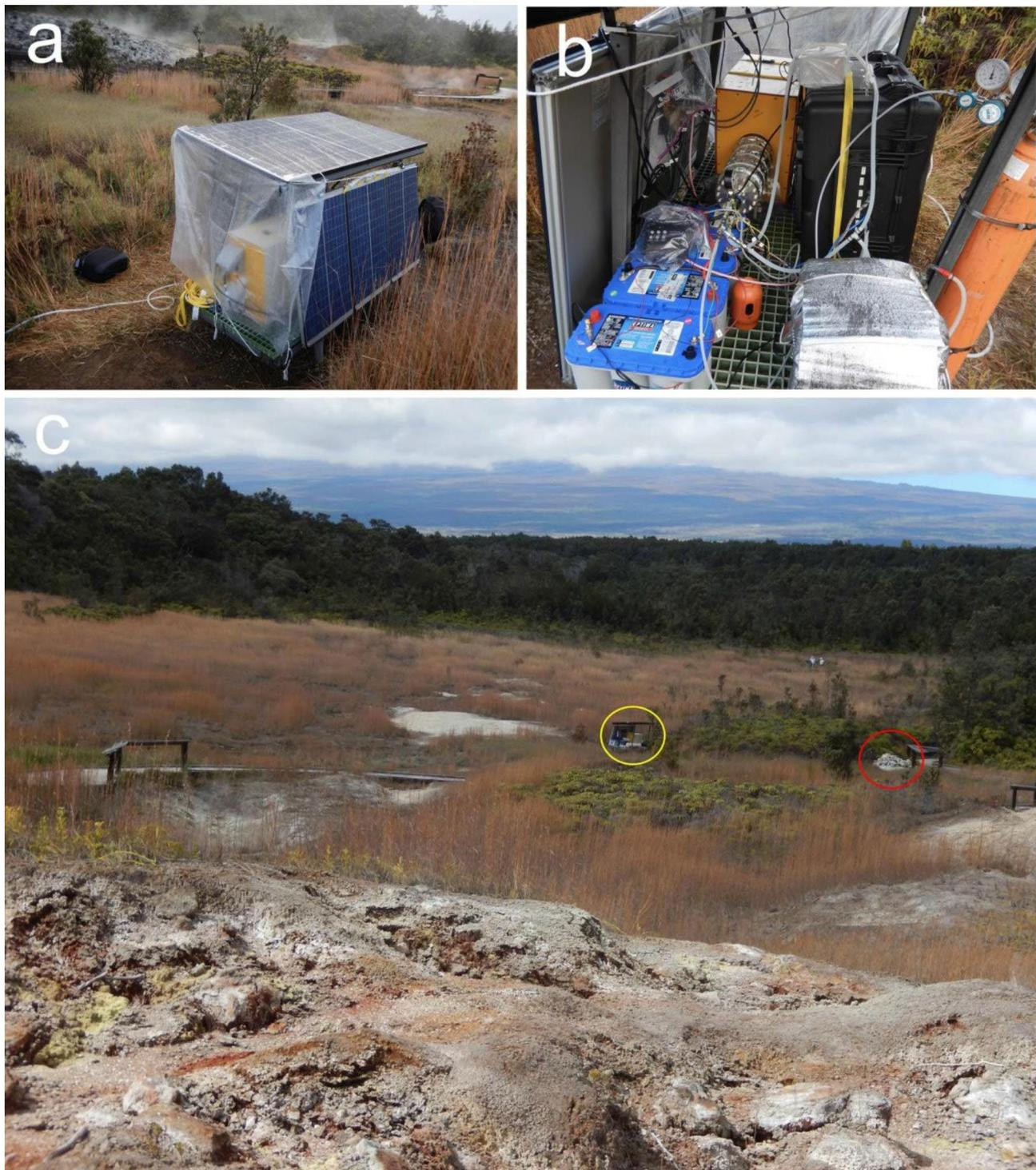
**Fig. 2** Photographs of the December 2020 deployment. **(a)** Solar-power equipped HIM Station with additional rain protection, looking east. **(b)** Internal layout (see text for detailed description of components). **(c)** Wide view of Sulfur Bank, looking NW. The Old Well fumarole is circled in red and the HIM solar station, which is located approximately 9 m S-SE on bare ground, is circled in yellow
